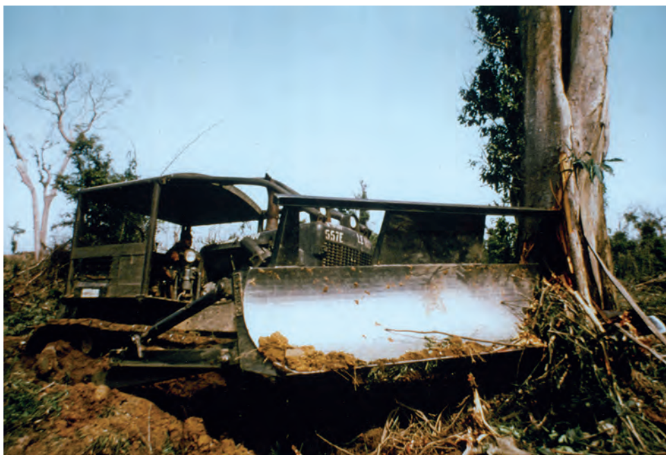
A modified D7E bulldozer equipped with a Rome plow and an armored cab
